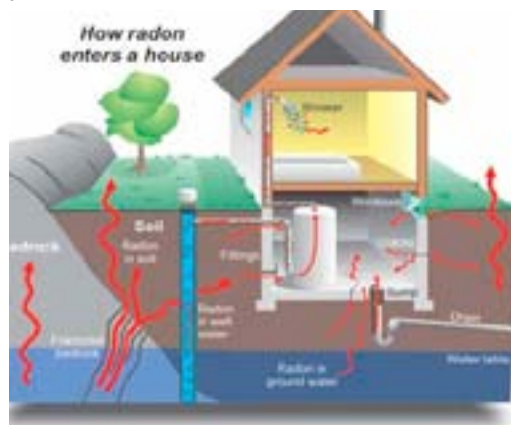
Figure 1: Radon entry locations.
