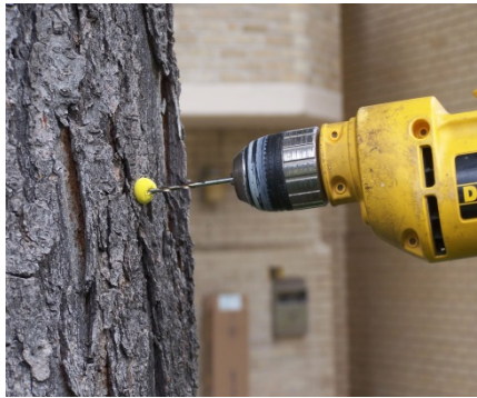
Figure 17. Examination of the sawdust and the pressure to push the drill through the annual growth rings give the experienced arborist a handle on internal decay. The yellow earplug on the drill bit helps the arborist know the depth as he works the drill bit in and out. With experience, the arborist could estimate percent shell for the spot drilled.
